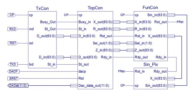
Fig. 8. FPGA structure of the enhanced logistic, enhanced sine and enhanced tent maps generated by SCM.
